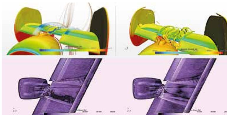
FLOW FIELD AROUND THE ENGINE/WING JOINING (ABOVE);
